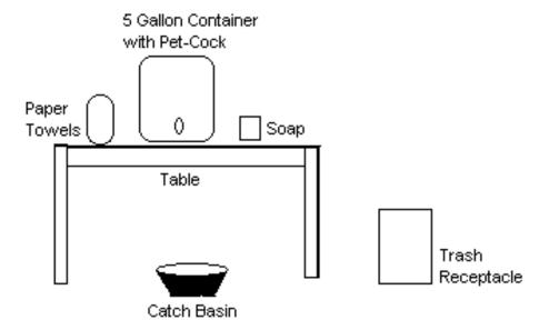
The most common cause of contamination during food preparation and serving is unclean hands. For this reason, hand washing facilities are a must. Facilities must be designed to provide unaided, easy hand washing under a continuous flow of running water. Water spigots of the push-button type will not be allowed.
